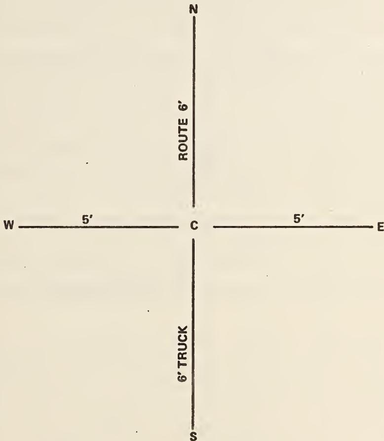
Figure 3.12 Soil Moisture Sampling Grid Pattern Used For Galena Line C'
